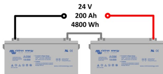
Two batteries in series.
