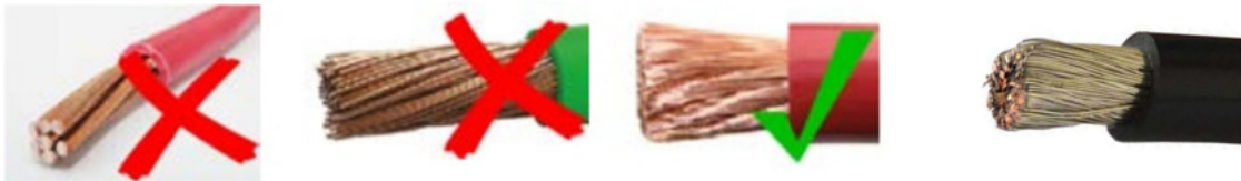
From left to right: non-flexible cable, cable with coarse strands, correct cable with fine strands, correct marine cable with tin coated strands.
